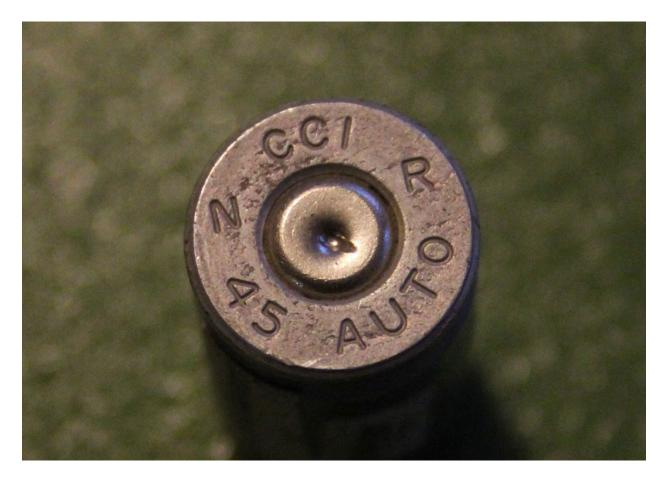
The primer of a centerfire cartridge is round and located in the center of the cartridge head. The firing pin of the firearm chambered for centerfire cartridges are either pointed or shaped like a punch. When the trigger is squeezed, the firing pin strikes the primer in the center of the cartridge head, which ignites the primer.
