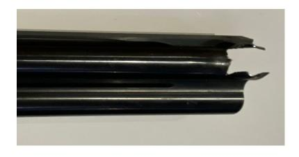
As a rule, never, ever, shoot steel shot out of a standard full choke or an extra-full choke, like used in turkey hunting. All full chokes and larger should be reserved for lead shot only. Also be aware of marketed chokes that can weaken the barrel of your shotgun resulting in a ruined barrel.
