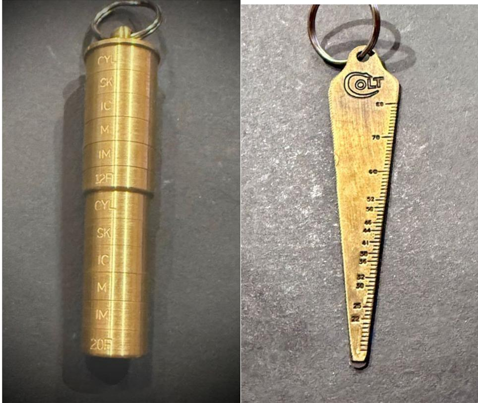
A bore gauge is used by inserting this instrument through the muzzle and taking a measurement in the barrel, behind the choke before the constriction starts. The second measurement is taken in the choke at the point of most constriction. The difference between these two measurements will give you the exact constriction of your choke.
