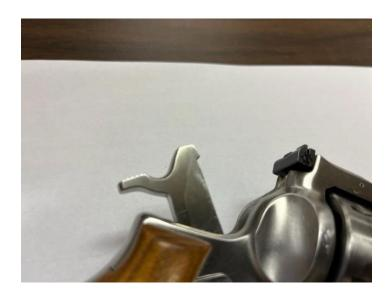
**Integral Fixed Firing Pin** – Integral firing pins are revolver fixed firing pins that are attached to the hammer and are a solid, non-moving component that impacts the primer of a cartridge or shotshell.
