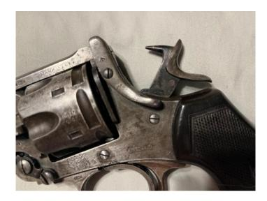
**Passive Firing Pins** – Passive firing pins are detached from the revolver's hammer and remain in the frame of the firearm. This type of firing pin is usually found in revolvers with a transfer bar safety system. In revolvers with a passive firing pin, the hammer swings forward, striking the firing pin in the frame, sending it to impact the primer of the cartridge or shotshell.
