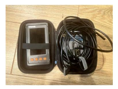
Bore scopes are great tools to use for inspecting barrels, chambers, and other hard to see areas. Bore scopes have a monitor and a flexible optic cable with a camera. Most optic cables have lights around the camera to light up dark areas. This is useful in looking for obstructions or damage in the barrel rifling that could affect accuracy.
