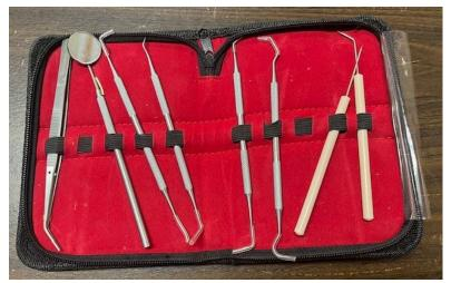
Brushes and picks are essential in getting at hard-to-reach residue, dirt, and grime. Brushes can be made of steel, bronze, or nylon. Steel and bronze brushes should only be used on metal parts. Nylon brushes can be used on all parts. Brushes are great for removing residue around the forcing cone of a revolver or cleaning the bolt face.
